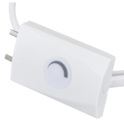
R2-PC3-FADE 20" power cord 5-100% control (hold) or 4-level control (tap)
